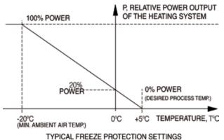
Performance characteristics are set by inputing the desired process temperature and the minimum anticipated ambient temperature, eg:  $-20^{\circ}C = 100\%$  and  $+5^{\circ}C = 0\%$  - as shown in the illustration. POWERMATCH MICRO + calculates the required temperature/energy profile.
