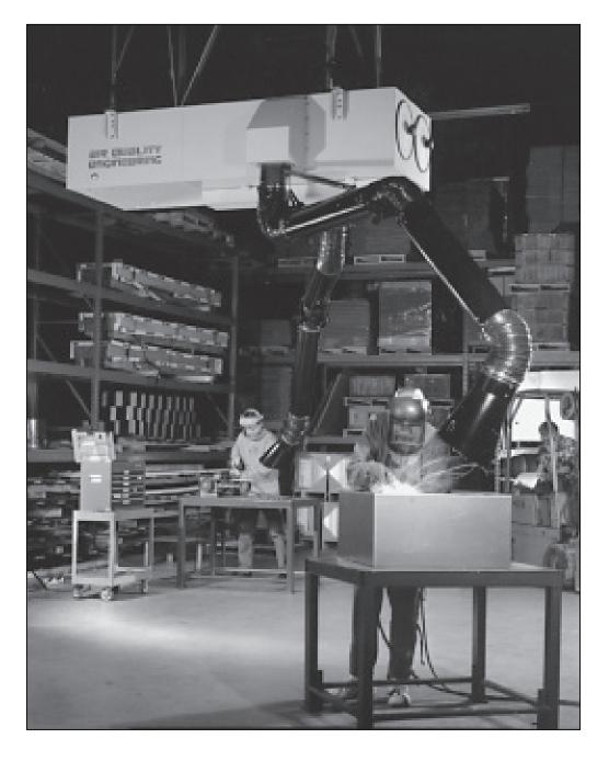
The new Overhead Cartridge System from Air Quality Engineering Inc. is a self-contained, continuous-cleaning cartridge media air cleaner for use in source capture applications in industry. The Model AQE4000 can be ordered in one and two arm configurations or permanently ducted to capture contaminants such as welding smoke, grinding dust, plastic dust and other fine particles.
